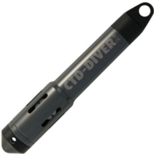
CTD diver : presure, temperature and conductivity sensor (Van Essen instruments)
